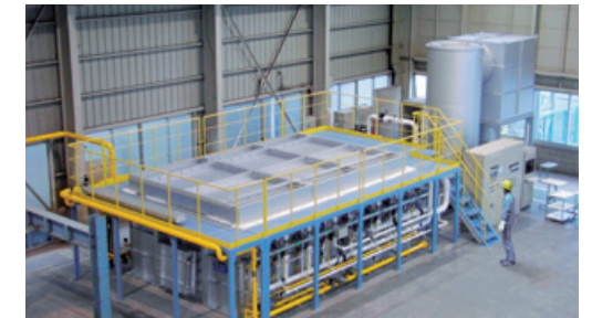
Fire resistance testing unit (horizontal furnace)
