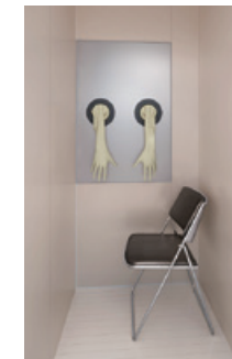
A partition with an opening for the use of gloves to perform tests
