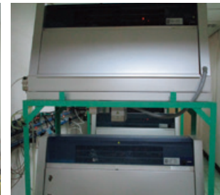
QUV weathering tester
