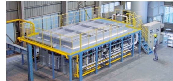
Fire-proof and Fire-resistance Test Equipment (Osaka Plant)
