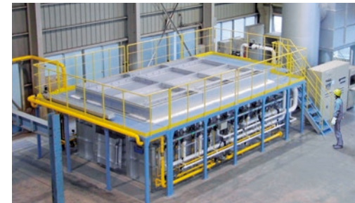
Fire-proof and Fire-resistance Test Equipment (Osaka Plant)
