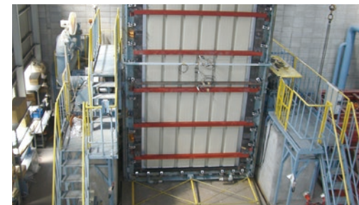
Water Spray and Air Blast Test Equipment (Osaka Plant)
